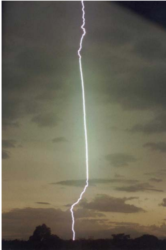
Fig. 5. Triggered lightning by LRSA technique. (Photo. O.Pinto/INPE)
