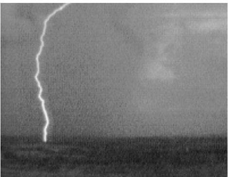
Photo 1 : t = d . Note the two forks, most likely emanating from the same charge pocket; the glow at the end of the stepped leader can clearly be seen on the right-hand fork..
